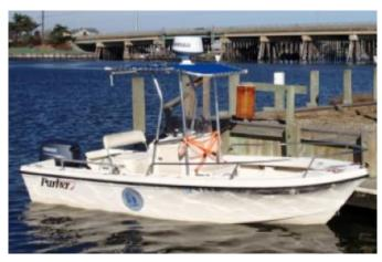
The Little Hawk is a versatile, trailerable, 18-foot fiberglass hulled center console survey vessel. The Little Hawk can be rigged to support a varity of scientific work including single and multibeam hydrography, sub-bottom profiling, side-scan sonar, ADCP surveys; benthic, fisheries and water column sampling along the coast.
