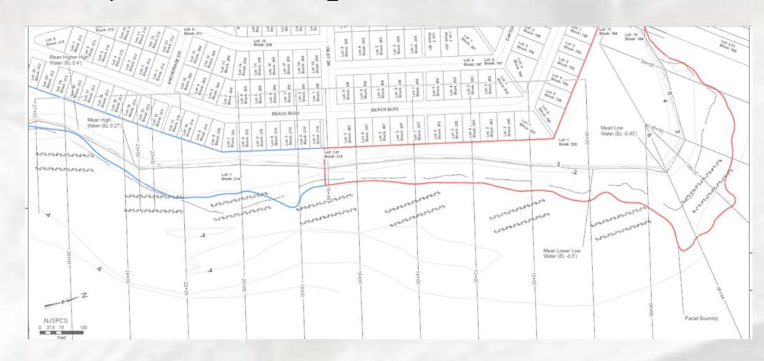
Each reef will be approximately 200 feet long and consist of a double row of 26 reef segments (13 in each row) arranged in a sawtooth-like pattern.
