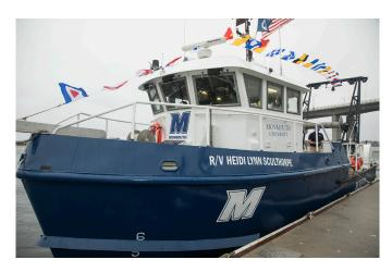
Acquired from NOAA and originally built as a Coast Guard buoy tender, the Research Vessel Heidi Lynn Sculthorpe is fully-equipped to operate up to 20 nautical miles offshore. The 49-foot vessel is rigged to carry out a variety of scientific operations, such as:
