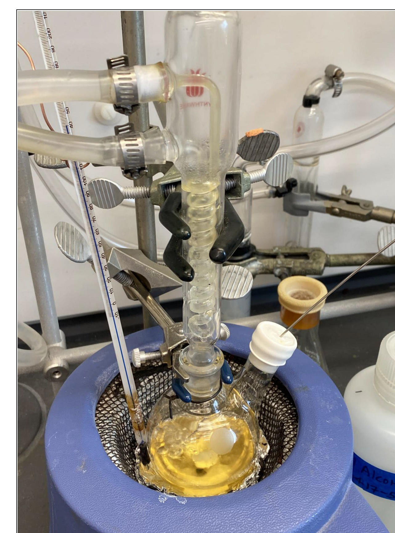
Figure 6. Reflux setup for the synthesis of a rhenium complex.
